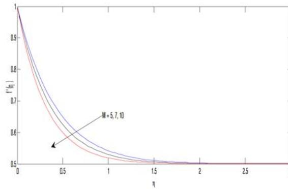
**Figure 3.** Velocity profiles for  $M$ .
